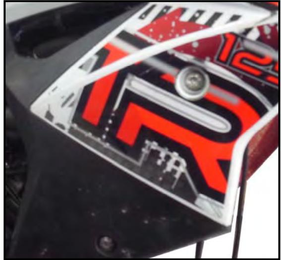
Disassemble gusset plate of right and left fuel tank
