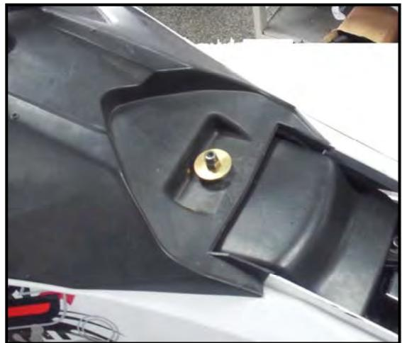
Disassemble air filter cover; fix bolts; take down the cover.
